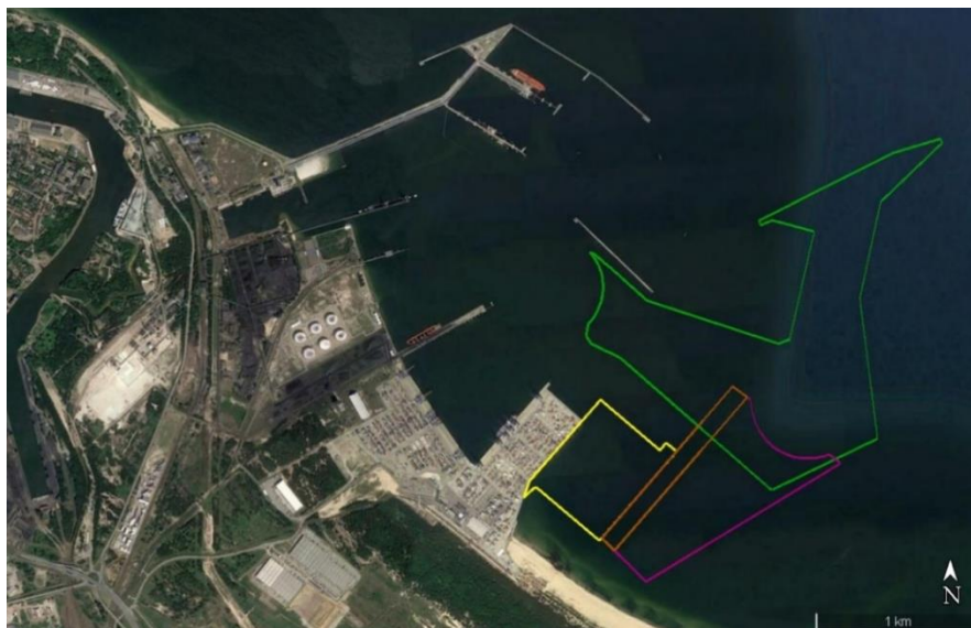
Figure 1.4: The location of the proposed T3 terminal (yellow), dredging for the T3 berthing area (purple), berthing area buffer zone (brown) and approach channels and turning circles (green).
