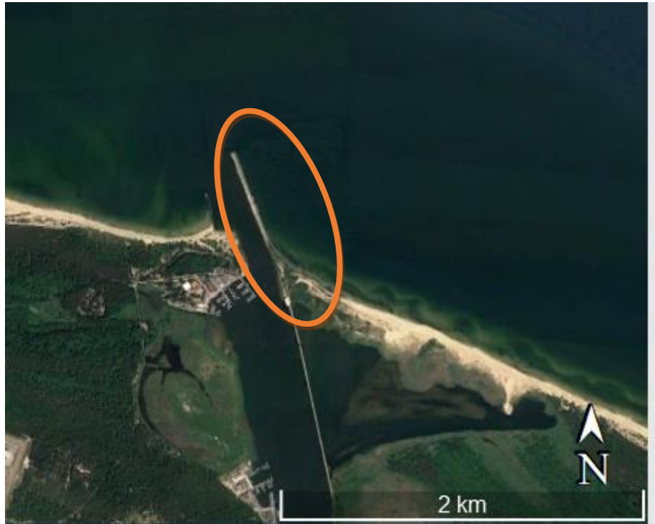
Figure 5.8: The mouth of the Marta Wisla showing no notable fillet on the eastern training wall.
