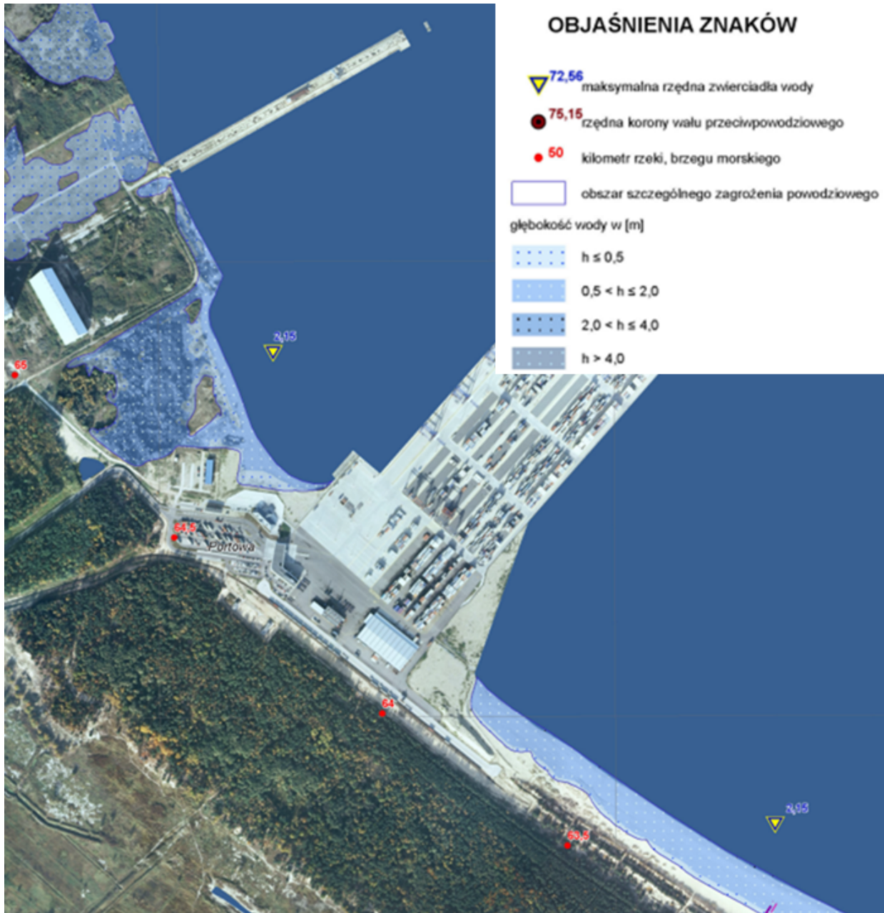
Figure 115: Seaward flood hazard map, including internal marine waters. Areas where flood probability is moderate and occurs once every 100 years (Q 1%). Gdańsk – Port Północny, N-34-50-C-d-2
