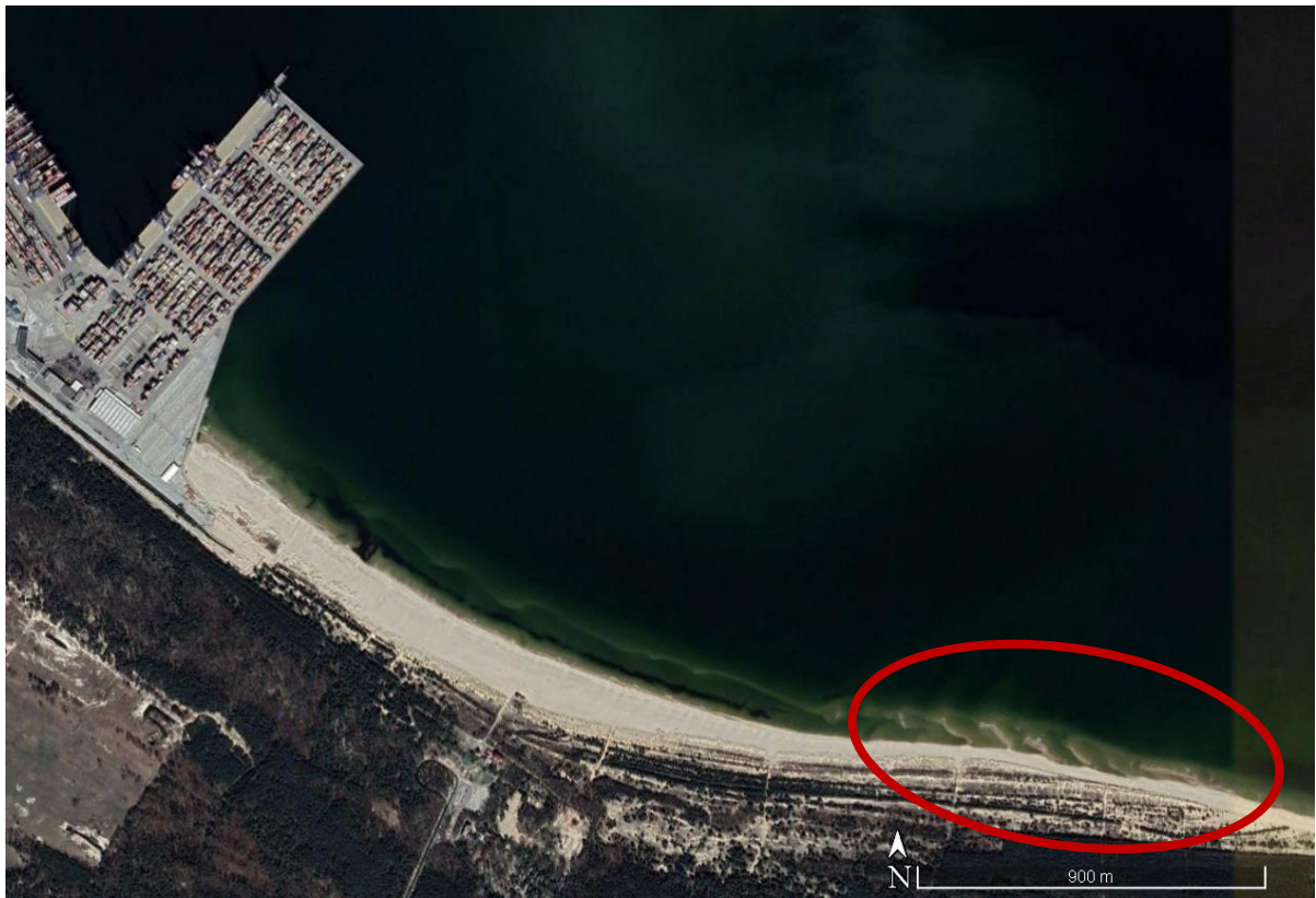
Figure 5.5: Ephemeral emergent bars that observed along the central section of Stogi Beach.
