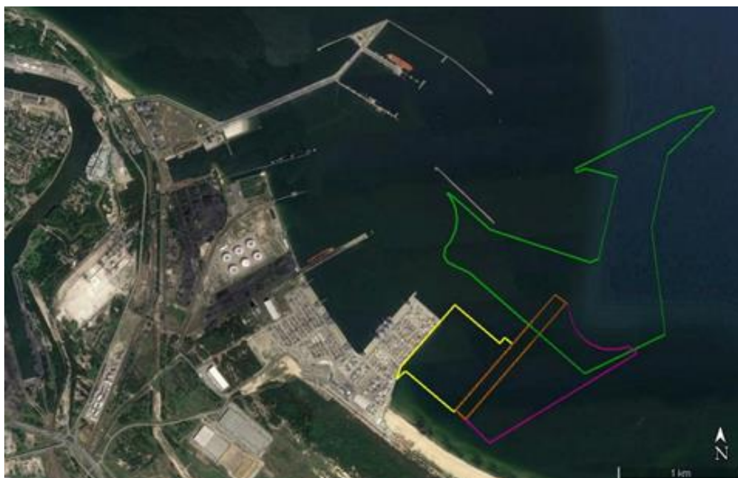
Figure 2 The location of the proposed T3 terminal (yellow), dredging for the T3 berthing area (purple), berthing area buffer zone (brown) and approach channels and turning circles (green).
