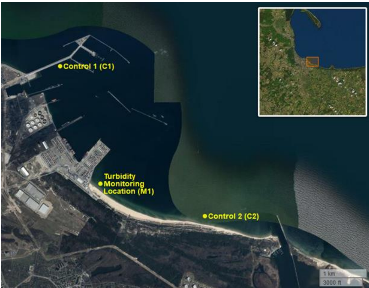
Figure 3 Turbidity monitoring location (M1) and two control locations (C1 and C2)
